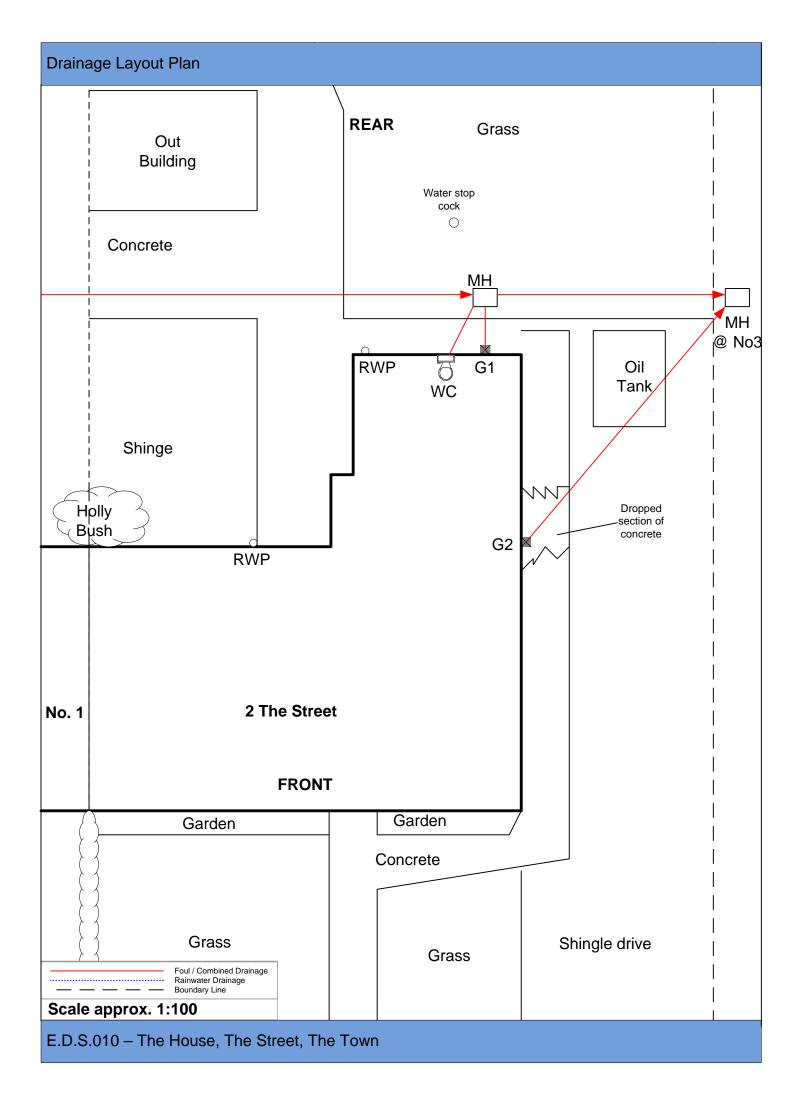
A shared drain runs from left to right across the rear approximately 0.5m from the rear building line. The private branch drains all join via manholes within the boundary or via the manhole at the neighbouring property (No. 1 The Street).
